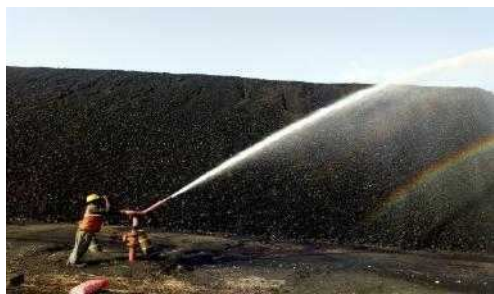
Water Sprinkling on Coal Hip
