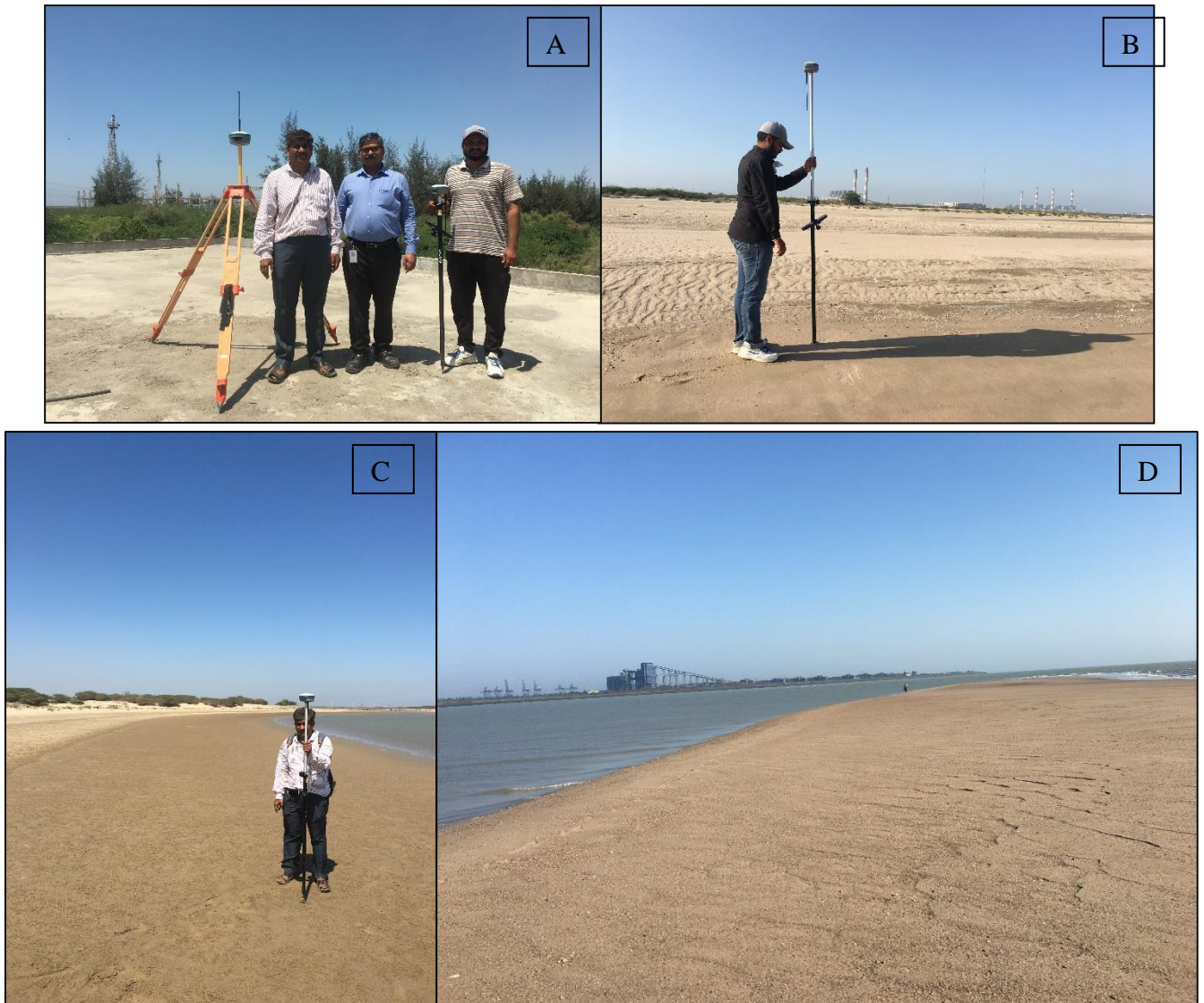
Figure 3.5: Establishing DGPS Base Station (A) And Collecting Survey and Ground Truthing Data(B), (C), (D) Using Rover.
