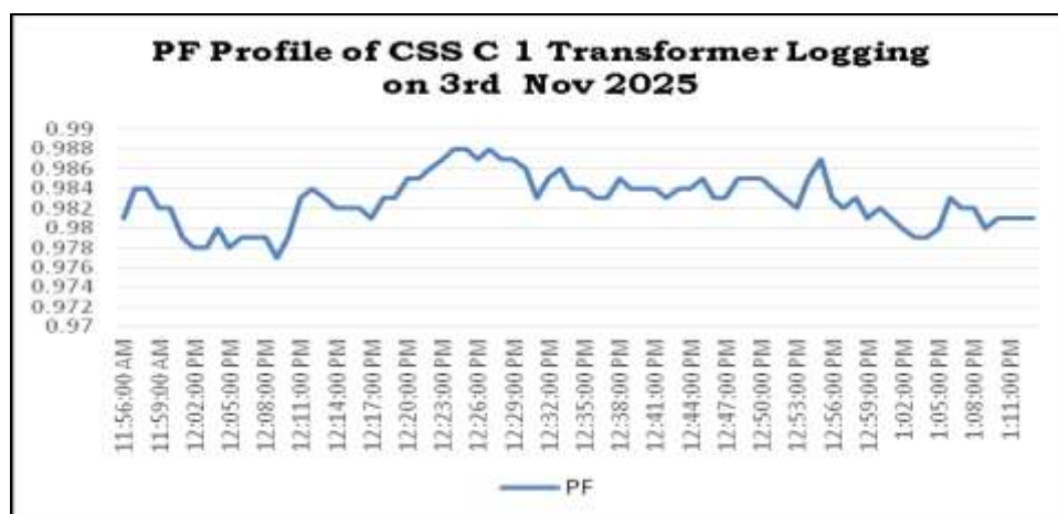
Figure 27 : Cos \phi T (DPF) Profile of CSS C1 1000KVA Transformer Main Incomer (Logging on 03rd Nov 2025)
