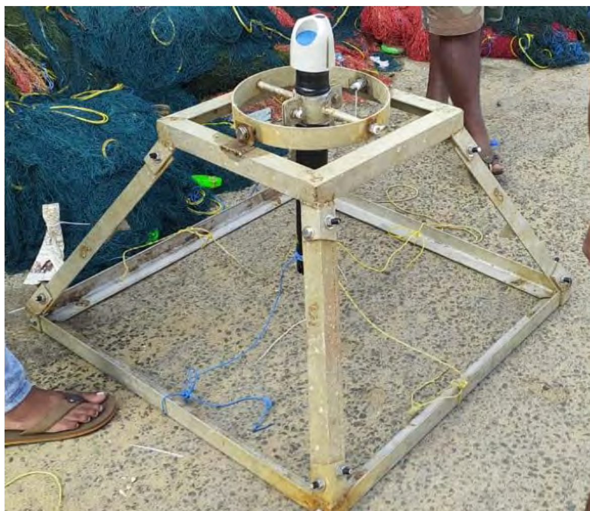
Figure 5-3: ADCP deployment at Vizhinjam
