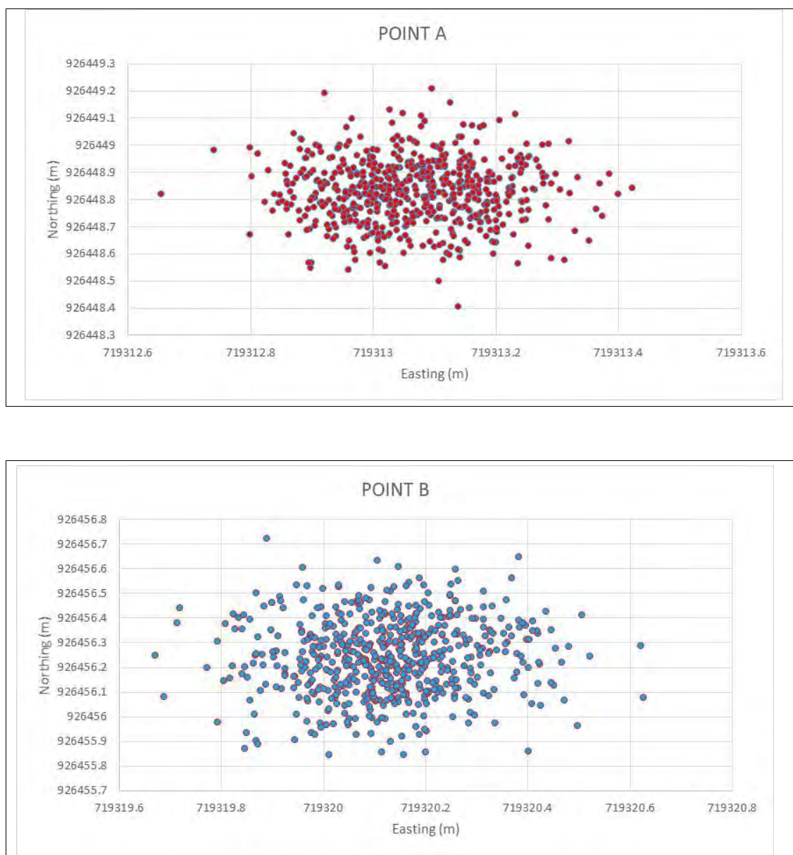
Figure 5-11: Scatter Plot of DGPS calibration on board M.F.B. Bethel
