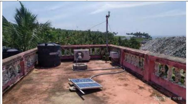
An image of automatic weather station is provided below:
