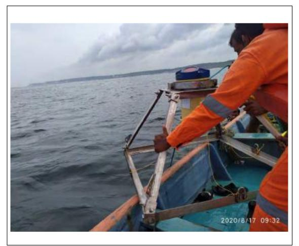
Figure 5-3: ADCP deployment at Vizhinjam by diver
