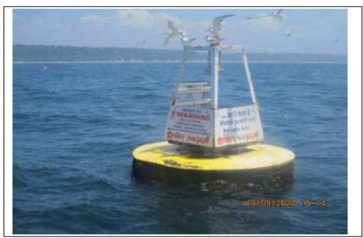
Figure 5-14: Turbidity Buoy
