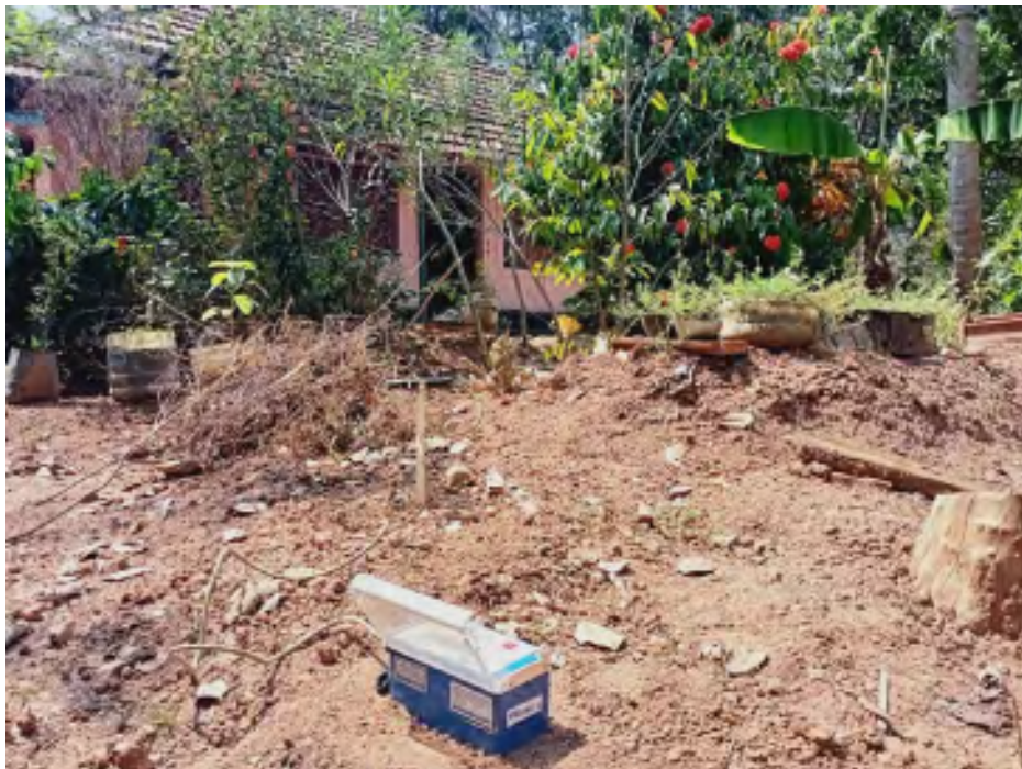
The monitoring instrument (S5) is located at the distance of 282 m from the blasting site (B4)
