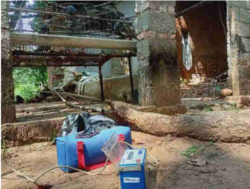
The monitoring instrument (S5) is located at the distance of 282 m from the blasting site (B8)
