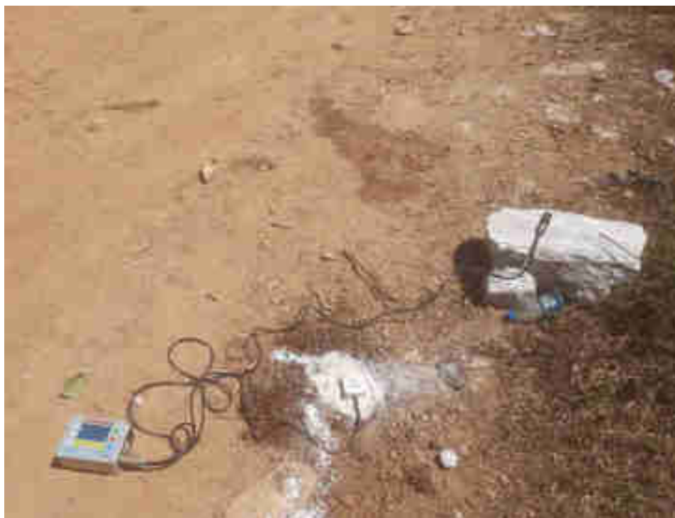
The vibration monitoring station (S1) is located at the distance of 297 m from the blasting site (B2)
