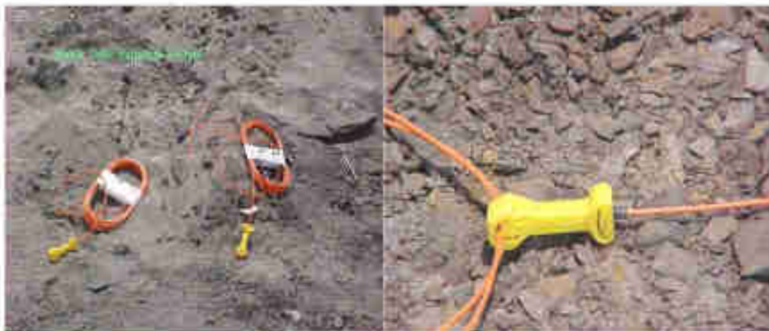
Figure 1.5 Non- Electric Shock Tube Initiation Systems
