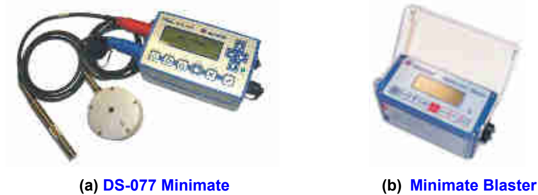
Figure 1.1 INSTANTEL Vibration Monitoring Instruments
