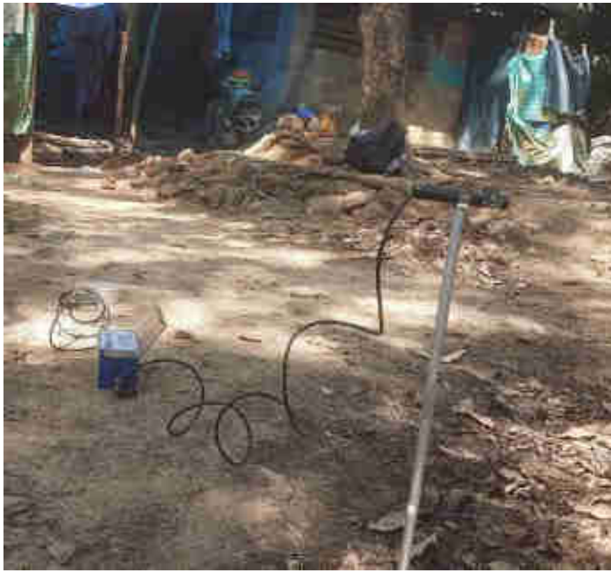
The monitoring instrument (S3) is located at the distance of 174 m from the blasting site (B6)
