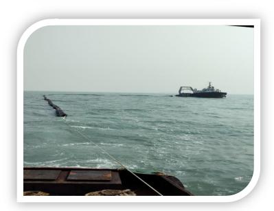
**1045 hrs.:** Skimmer deployed in water. The floating storage tank was kept ready on Dol 11 deck. The Overside OSD spray was pressurized and demonstrated with water only.
