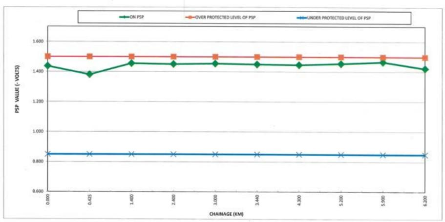
As per criteria for PSP as per OISD 226 / 12.3.5 A or NACE SP0169-2013 measured wrt Cu-CuSO4 reference Electrode, the subject pipeline section is cathodically protected. Hwoever, for true potential, OFF PSP shall be measured once a year.
