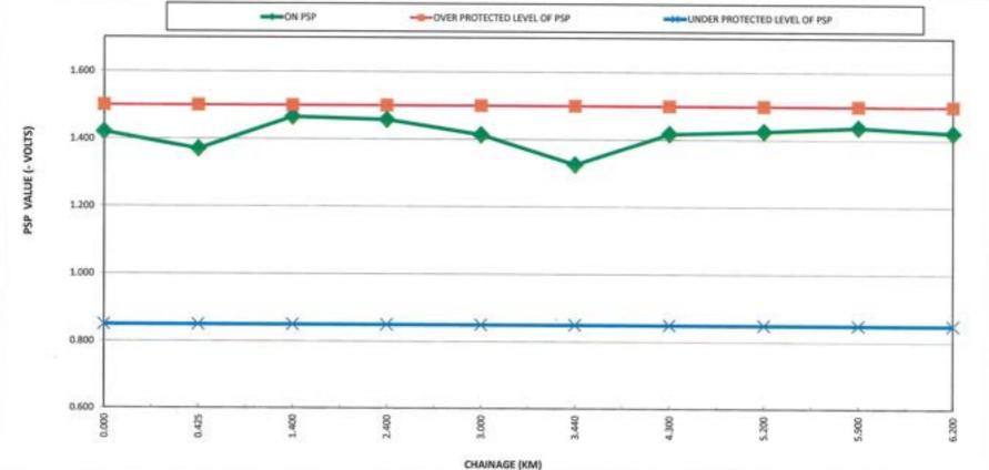
As per criteria for PSP as per OISD 226 / 12.3.5 A or NACE SP0169-2013 measured wrt Cu-CuSO4 reference Electrode, the subject pipeline section is cathodically protected. Hwoever, for true potential, OFF PSP shall be measured once a year.
