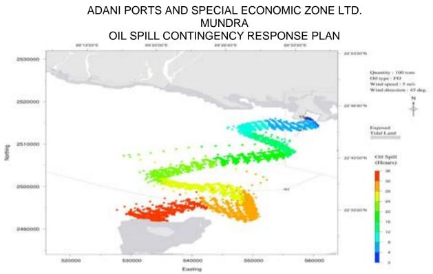
Oil Spill trajectory due to instantaneous FO leakage of 700 t (due to hull failure/ fire / explosion) at typical berth location in the West Basin
