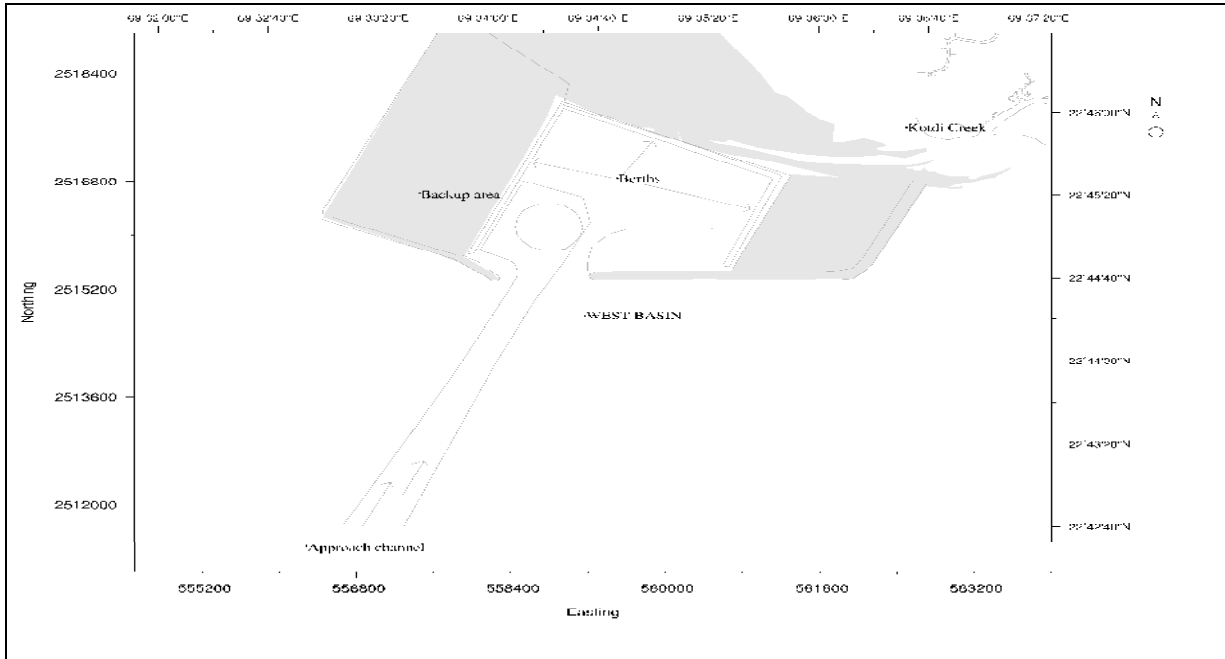
Fig.1.3 Zoomed up portion of the West Basin showing the berth locations and the approach channel for the vessels
