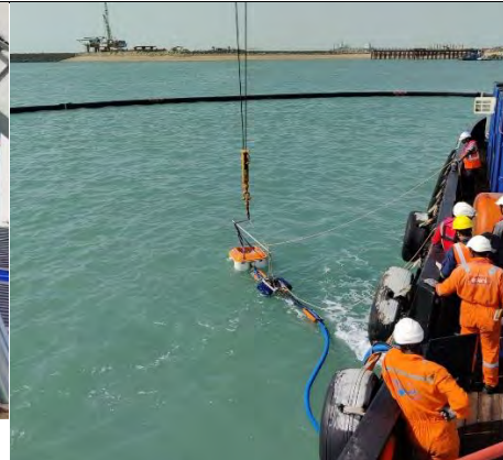
Collection of spilled oil by Skimmer
