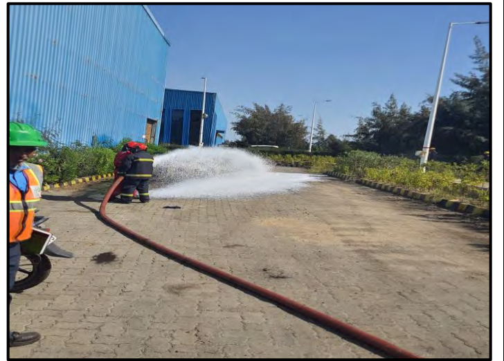
Fire-fighting Foam making by using FB-10 Branch from Foam Mobile Unit located / Installed at Central Store by water connectivity from Fire Hydrant network
