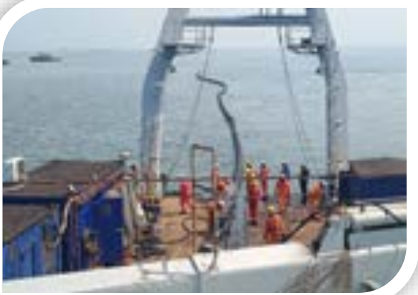
Lowering boom (5 section 250 m in length)
