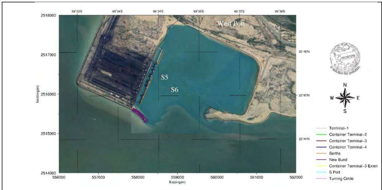
Fig.1.4 Zoomed portion showing marine facilities of West Basin and spill locations selected
