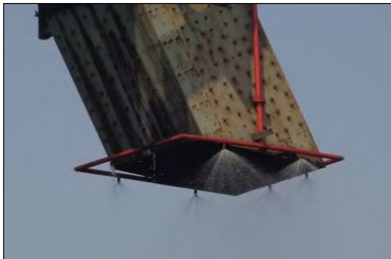
Coal Chute point having water Sprinkling System
