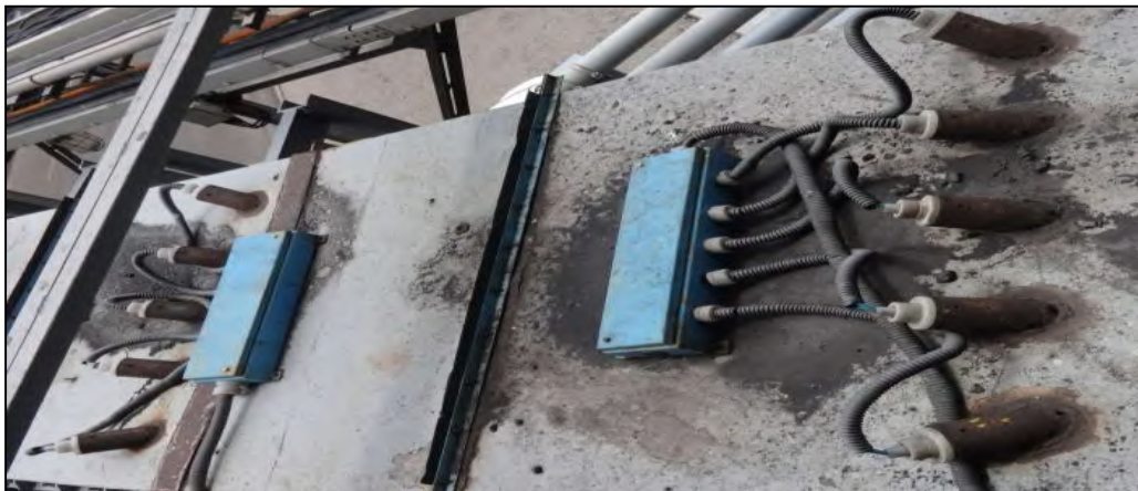
Dust Suppression System Installed in Conveyor System
