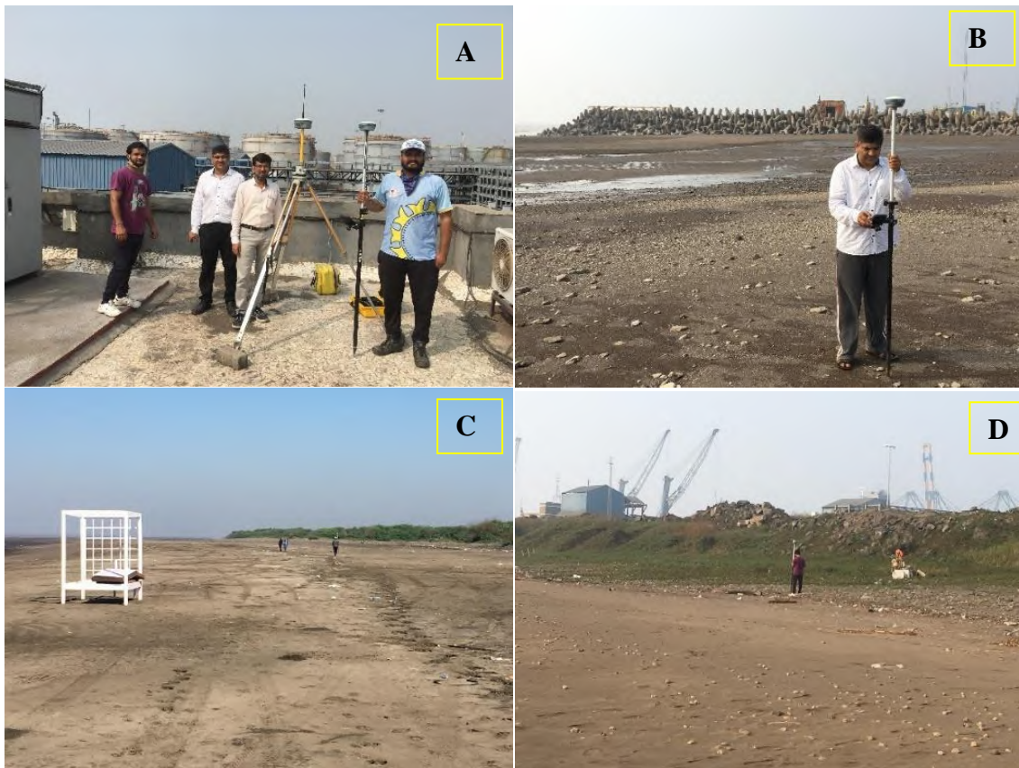
Figure 3.5: Establishing DGPS Base Station (A) And Collecting Survey and Ground Truthing Data(B), (C), (D) Using Rover.
