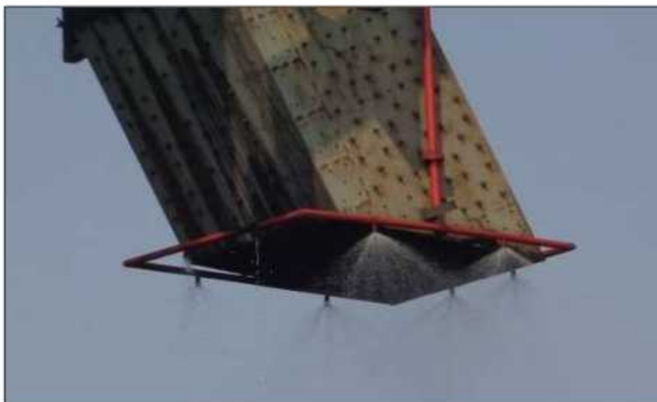
Coal Chute point having water Sprinkling System
