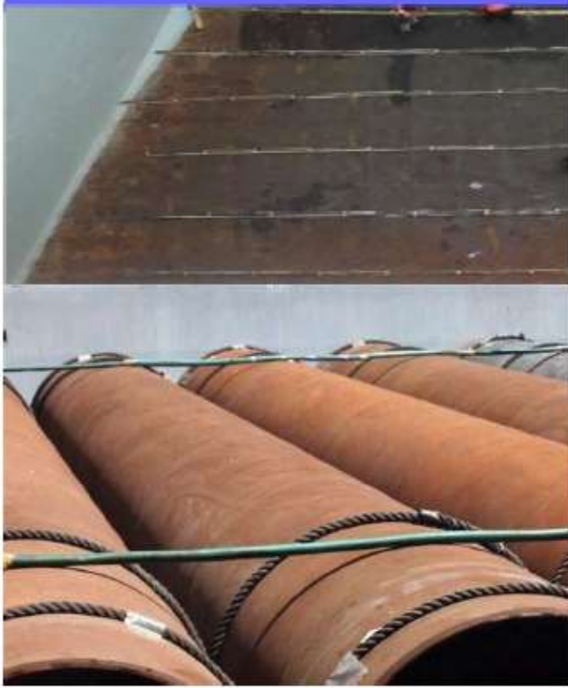
Picture of Dunnage Lines on Tank Top & Lashing Wires per Stack
