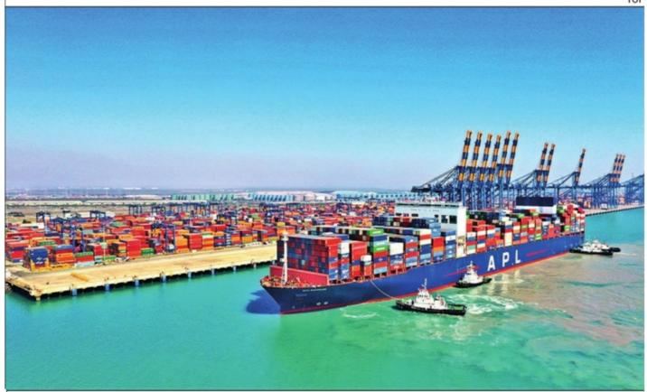
Mundra became the port to have berthed the largest container vessel in India when APL Raffles docked there on Friday. APL Raffles is registered in Singapore and is one of the biggest vessels in the fleet of French container transportation and shipping company, CMA CGM Line. It was built in 2013 and is 397.88m long, 51m broad and 76.2m high. It has a net tonnage of 76,852 tonnes.
